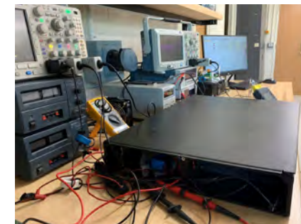
Online UPS inside a chassis for testing under practical conditions of a data center. Photo provided.
