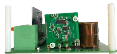
Side views of the proposed high power density online UPS prototype built in the lab, capable of achieving a power density of 26.4 W/in 3 . Image provided.
